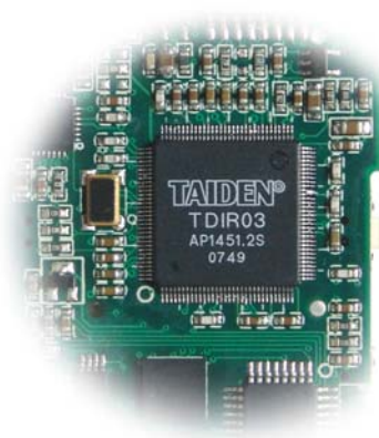
TAIDEN TDIR03 digital infrared processing chip
