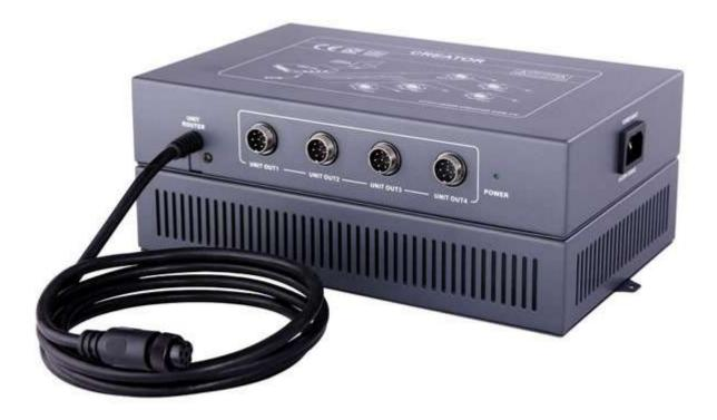
The CR-HMP24 power supply unit for conference system is used for the power supply extension of speech units. In case of host insufficient power supply, this device achieves the purpose of relay. It supports four unit outputs.
